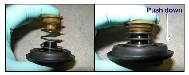
4. Select the appropriate number of shims from the list below. Remember, the CBV shims **do not increase the boost level of your vehicle**; they only allow the CBV to hold higher boost pressures without leaking! You can only increase the boost level of your vehicle through an ECU upgrade, boost controller, wastegate adjustment, etc. Count the shims according to the maximum amount of boost your vehicle normally runs at:
