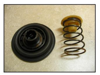
3. With the CBV diaphragm now disassembled, place the spring and seat onto the new CBV diaphragm, and snap the seat down onto the CBV diaphragm as shown:
